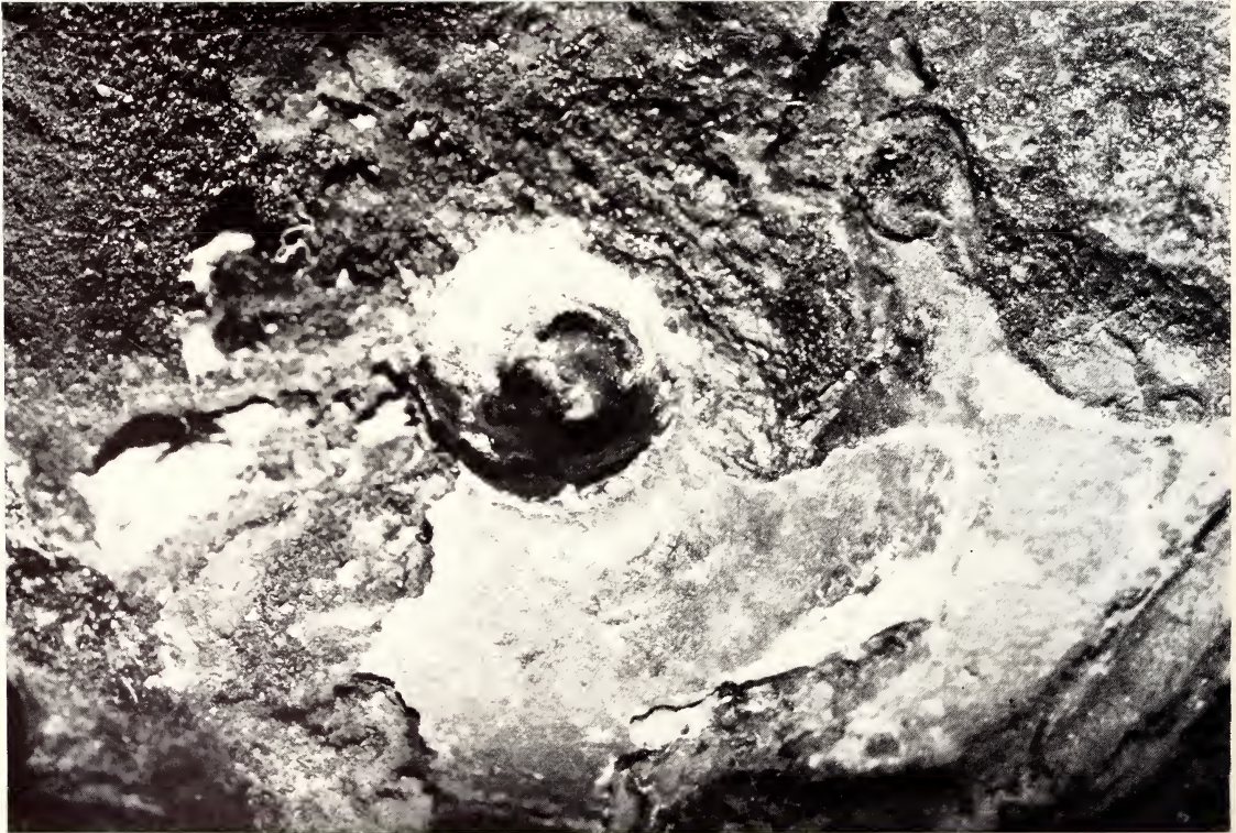
FIG. 14.—34.11. Chinese bronze dagger axe. The macrograph ( \times 9.2 ) shows a drill hole that was made near the end of the bronze blade passing through the outer encrustation of iron rust, through the bronze layer and into the inner iron core. After about five years in storage, a crusty brownish globular shaped deposit of ferric chloride formed in the drill hole.
